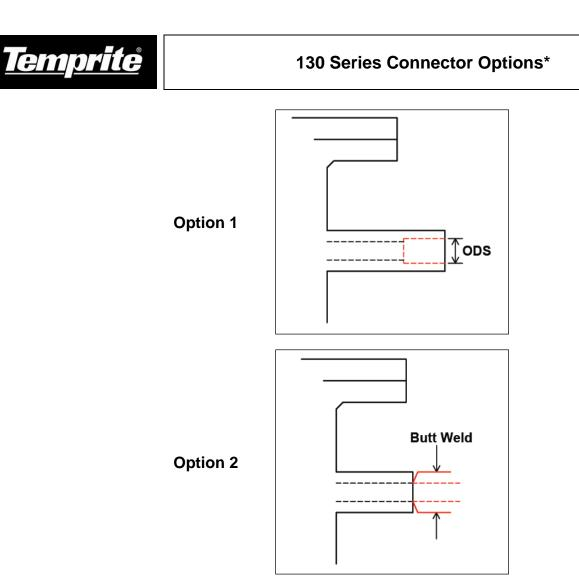
Option 2 requires the installer to cut off the excess ODS portion of the connector and then butt weld a pipe to the shortened connector. \*Not available for 139A (2")
