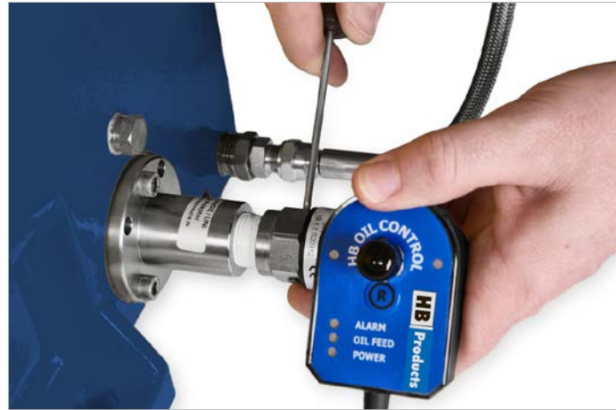
The sensor housing is re-installed, either via a mounting tab or it is secured with 2 grub screws.
