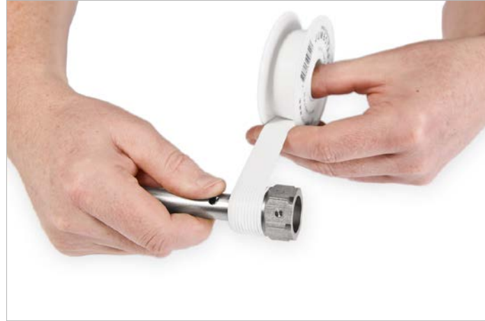
Teflon or liquid gasket is applied to the conical thread. Cylindrical thread is installed with gasket.
